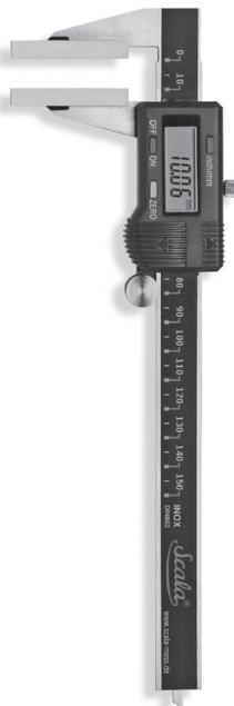
Wide flange calipers are specialized calipers designed to measure wire rope diameters. The flanges are wide so the contact spans over more than one strand to give an accurate measurement.
