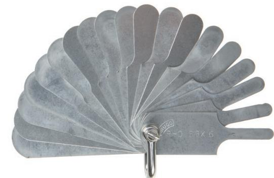
A radius gauge allows the technician to quickly determine if the sheave groove is worn. Seat the radius gauge in the groove and direct a flashlight at the radius gauge from behind where it is seated in the groove. If light can be seen under the radius gauge, the sheave groove is worn. To get the exact depth of wear, use the GDC.
