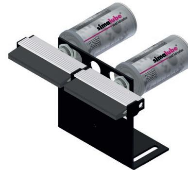
The Simalube Smart Lubrication device automatically releases the flow of metered field lubricant that is guaranteed compatible with the grease applied in the wire rope factory. The lube flow rate is set with an allen wrench to meter the flow of the lube over a customized period of one to 12 months.
